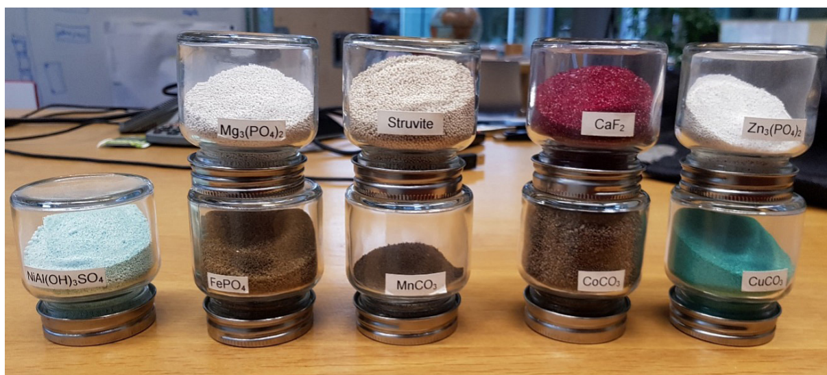
A range of minerals, including phosphorus-based products, can be recovered in valuable forms from municipal and industrial wastewater using Crystalactor technology
