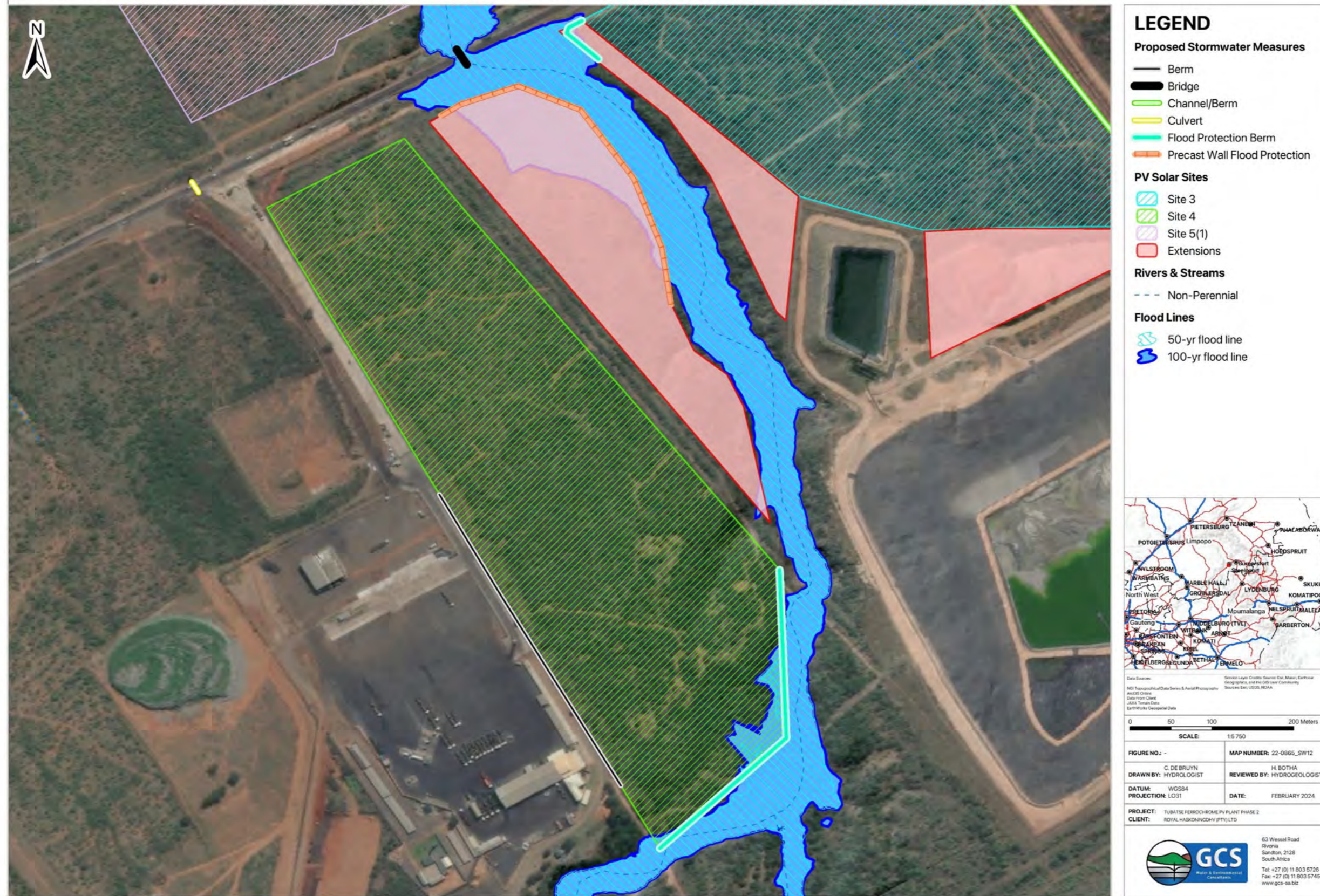
Figure 6-15: Proposed stormwater infrastructure for Site 4
