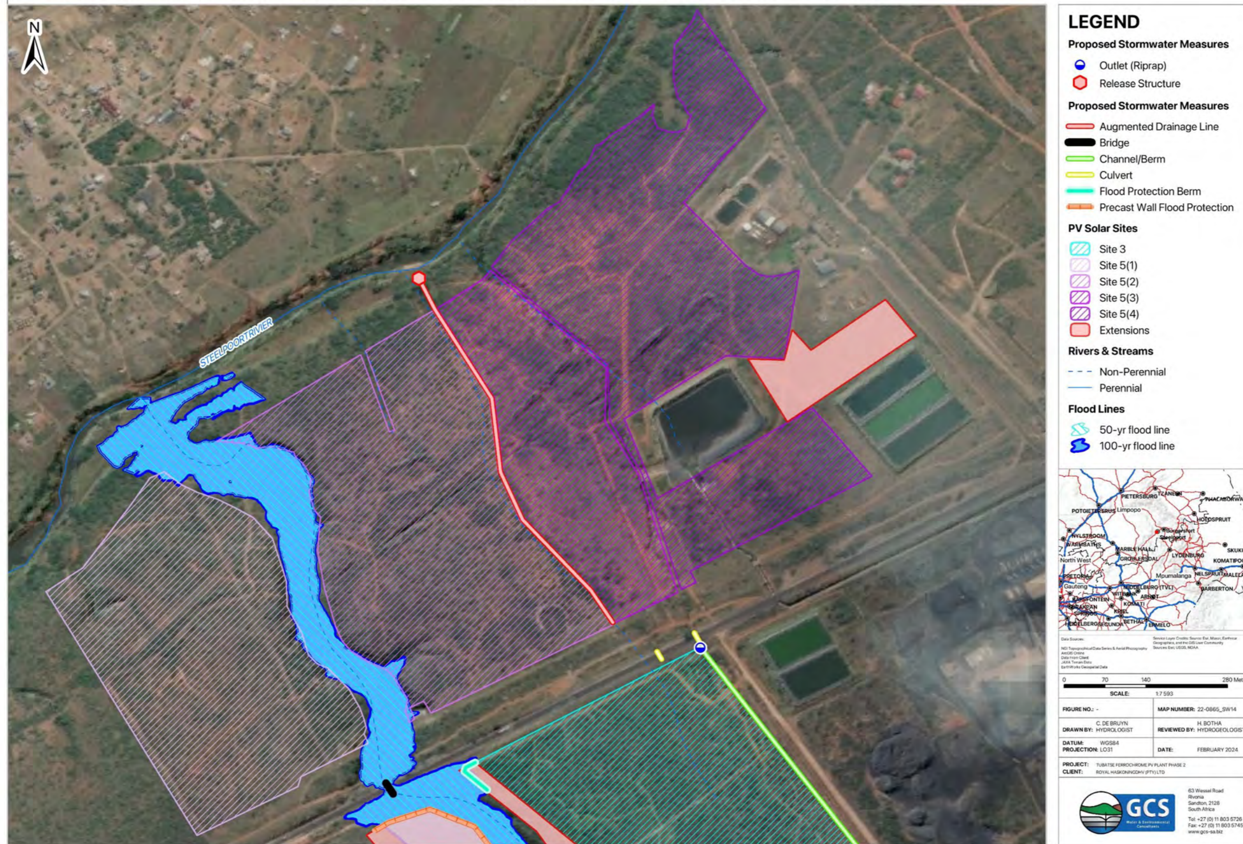
Figure 6-17: Proposed stormwater infrastructure for Site 5
