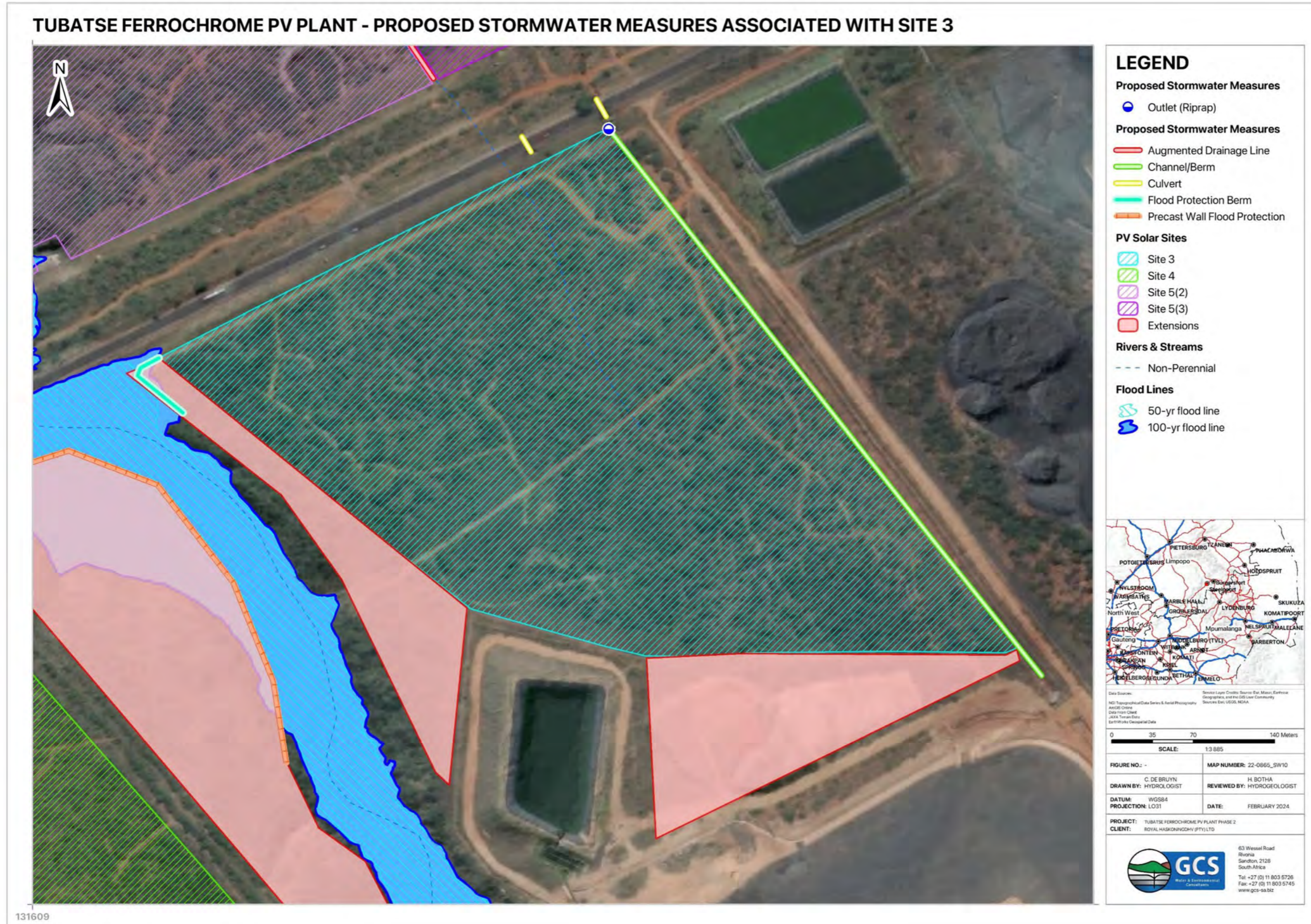
Figure 6-11: Proposed stormwater infrastructure for Site 3
